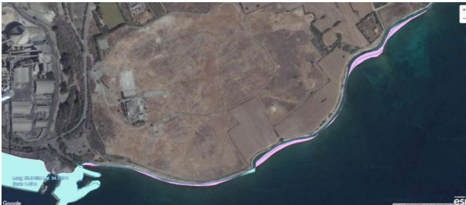
Figure 2-8. Erosion and accretion areas at the east side coast of the port (Department of Lands and Survey - Ministry of Interior). Pink color indicates erosion areas while light blue indicates accretion areas
